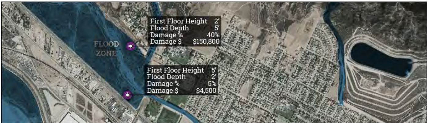
Figure 4-10: Hazus Damage Estimation Example
