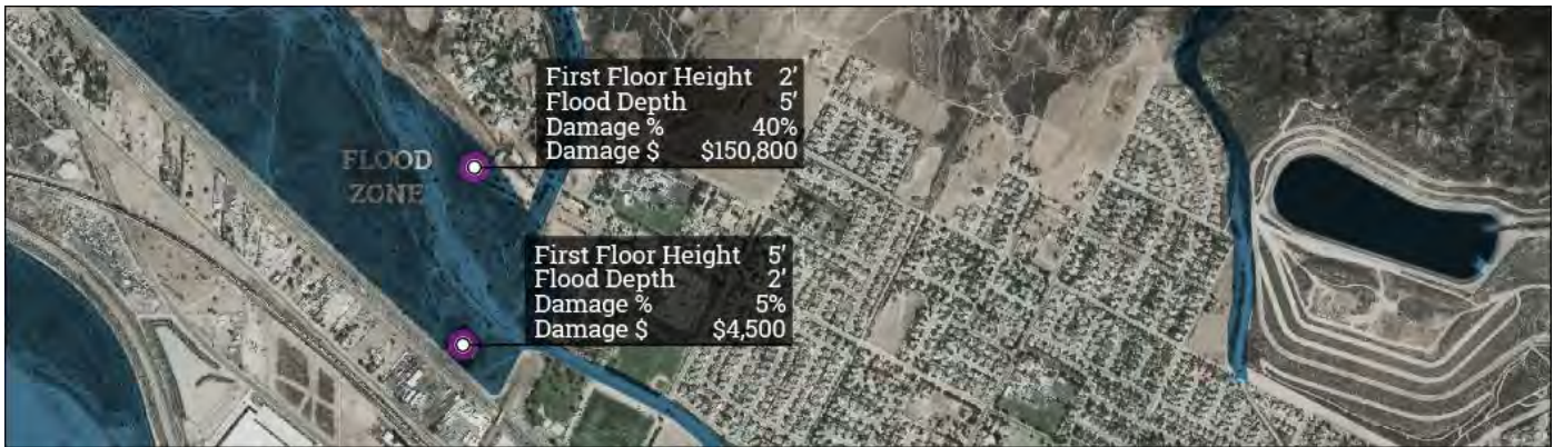
Figure 4-10: Hazus Damage Estimation Example
